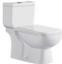
Code: 2341A 直冲式分体坐便器(横排) Washdown Two-piece Closet(P-trap) Size: 645×365×800mm S-trap: 220, 250, 300mm Roughing-in P-trap: 180mm Roughing-in
